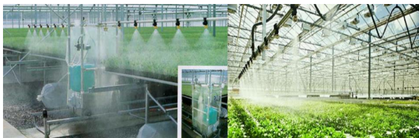
Figure 53: Overhead sprinkler systems as installed in greenhouses 164
