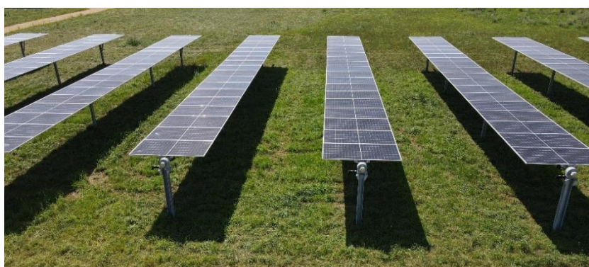
Figure 16: Single axis solar tracking system. 6
